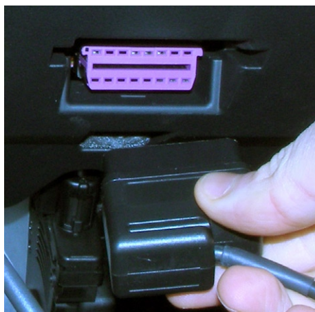
Fig. 4: A typical vehicle CAN connection.
