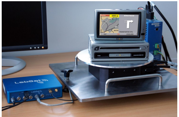
Fig. 3: A setup on a precision turntable can reproduce GPS heading to test the unit's gyro response.
